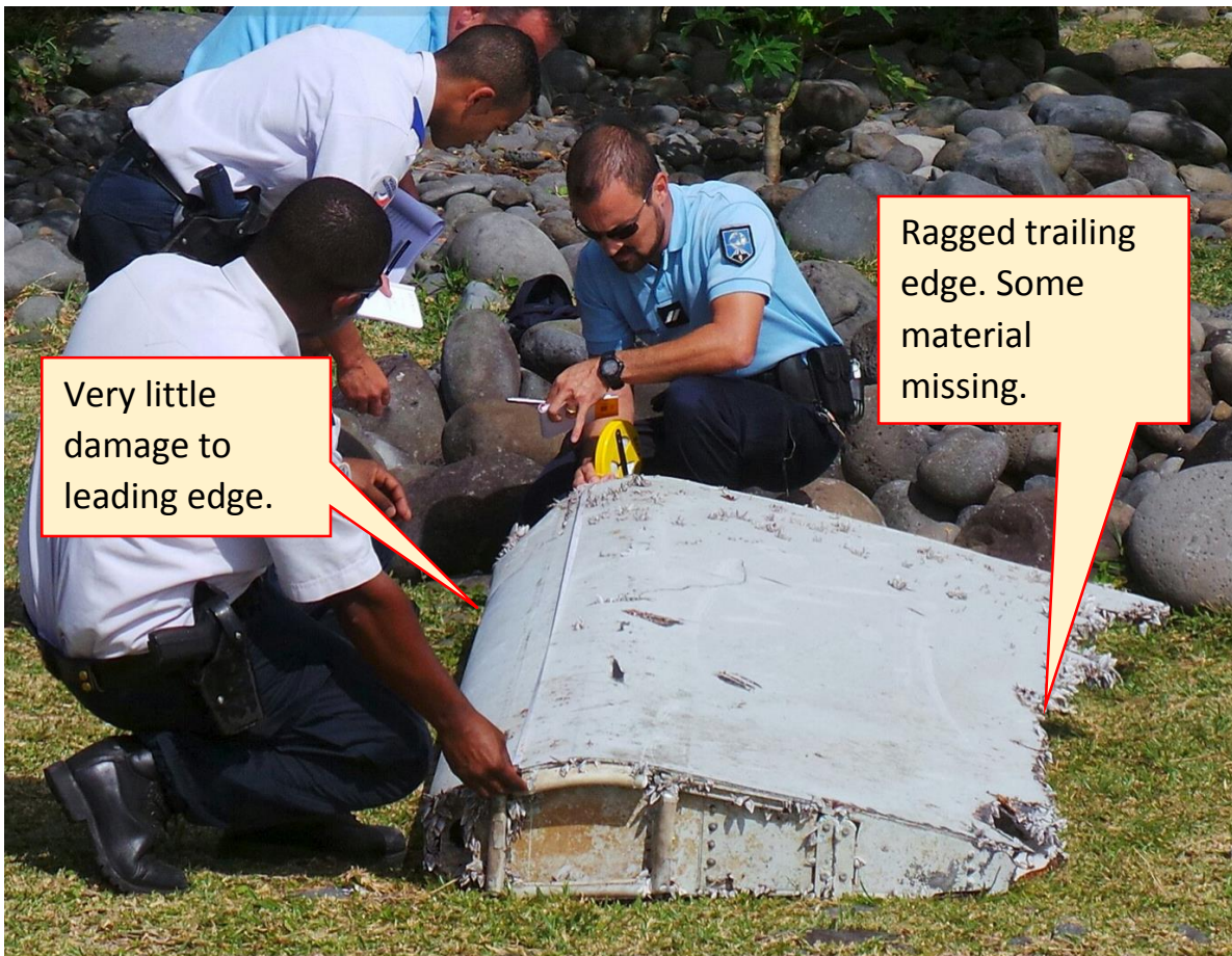
Debris found on Reunion Is. The shape, dimensions and P/Ns found on debris are consistent with a wing component from a B777 airplane, most likely the right “Flaperon” from MH370.
