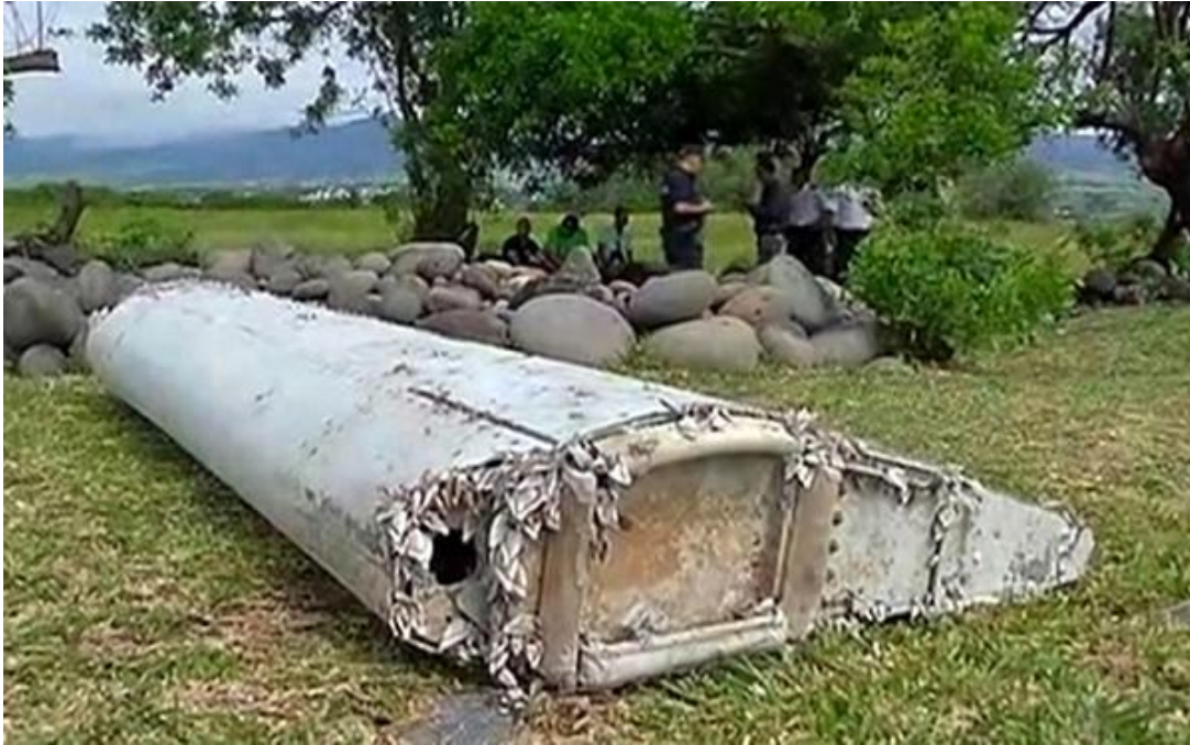
Left end of Right Flaperon (to be verified by serial number). Note lack of damage to leading edge.
